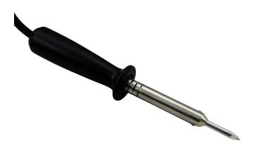
American Beauty heavy-duty irons are ideal for heavy soldering jobs and production-line environments. Created by compression winding a special Ni-Chrome heating alloy onto a steel spool, all elements demonstrate an unsurpassed heat capacity and outstanding durability. Protective casings cut from a single block of steel are strengthened with multiple heat treatments and precision brazed for optimal strength and efficiency. (*Stand Included*)
