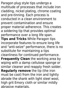
Return the tip to the iron after cleaning and ensure it is **fully seated** into the heating element.
