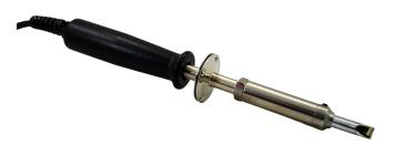
American Beauty heavy-duty irons are ideal for heavy soldering jobs and production-line environments. Created by compression winding a special Ni-Chrome heating alloy onto a steel spool, all elements demonstrate an unsurpassed heat capacity and outstanding durability. Protective casings cut from a single block of steel are strengthened with multiple heat treatments and precision brazed for optimal strength and efficiency. (*Stand Included*)
