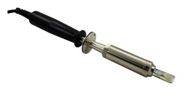
American Beauty heavy-duty irons are ideal for heavy soldering jobs and production-line environments. Created by compression winding a special Ni-Chrome heating alloy onto a steel spool, all elements demonstrate an unsurpassed heat capacity and outstanding durability. Protective casings cut from a single block of steel are strengthened with multiple heat treatments and precision brazed for optimal strength and efficiency. (*Stand Included*)
