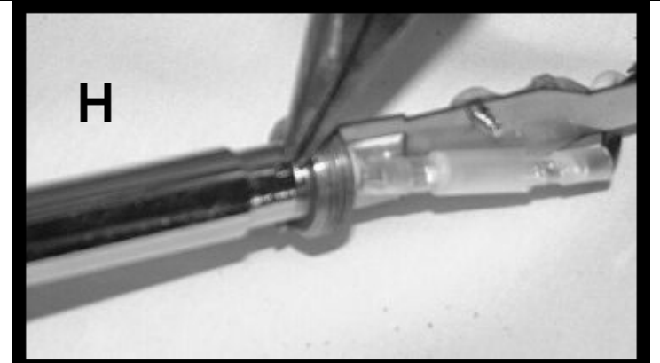
Secure in place via re-bending tabs. Re-tape strain relief assembly, slide wood handle back in place and hand tighten.
