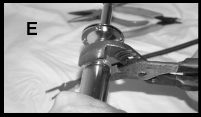
Loosen spanner nut. Expired heating element should slide freely from the soldering iron casing. Dispose.
