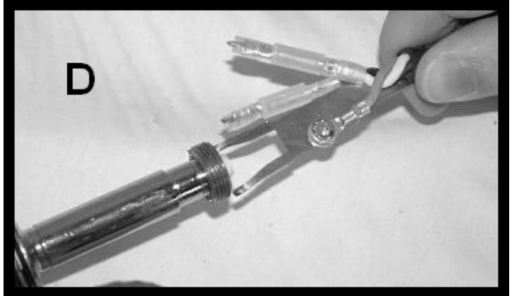
Gently remove cord set / strain relief assembly from soldering iron casing. Separate and discard male QCT's from the females.
