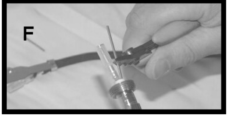
Insert new heating element and secure with spanner nut. Factory provides heating elements with longer electrical leads than required. Trim the leads (on angle) from the new element so that the provided male QCT's sit snugly against ceramic insulator. Crimp.
